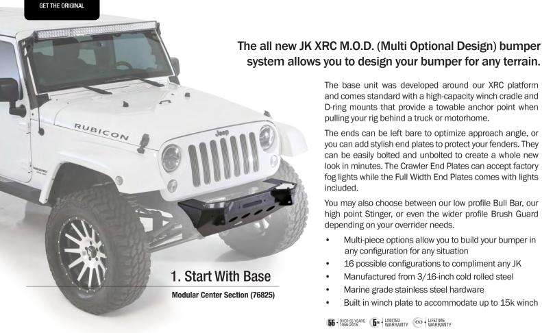
The base unit was developed around our XRC platform and comes standard with a high-capacity winch cradle and D-ring mounts that provide a towable anchor point when pulling your rig behind a truck or motorhome.
