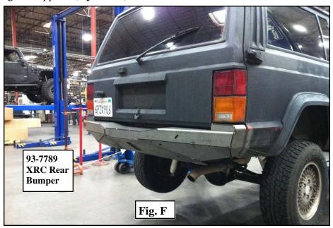
**Step 8:** Level the bumper and torque all mounting hardware according to the chart on page 7 or manufacturers specifications.
