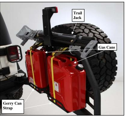
Step 27: With the tire gate fully loaded, adjust the cam wheel (90-9214) to make sure gate closes properly. Using a 3/8" ratchet, insert the ratchet into the cam wheel and rotate the cam wheel until it lifts the weight of the gate. Inspect and ensure the latch and striker mate properly. Once the striker and latch are aligned properly, install the 3/8" X 3/4" black Allen head bolt through the window in the cam wheel to lock it in place. Torque the 3/8" bolt to 18 ft./lbs. (Fig. P)
