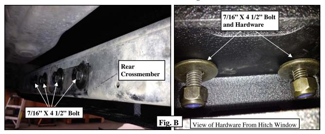
**Step 6:** Torque the **7/16**" bumper hardware to **55** ft./lbs. and **1/2**" hardware the **80** ft./lbs. (Fig B)
