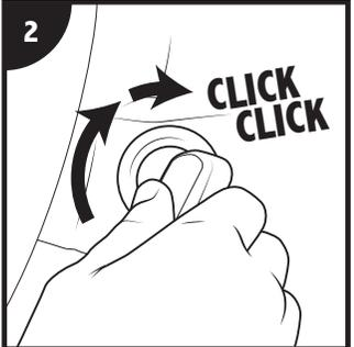
Insert the key into the ignition and turn TWO clicks to put the vehicle in the "run" position.
