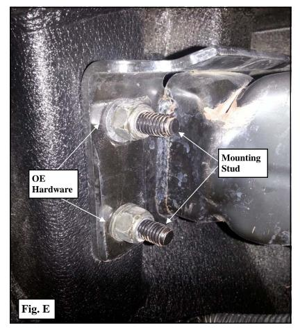
**<u>Step 11:</u>** Level the bumper and torque the **OE** hardware to manufacturer's specifications. (Fig E)
