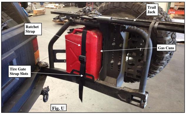
Step 33: With the tire gate fully loaded, adjust the cam wheel (90-9516) to make sure gate closes properly. Using a 3/8" ratchet, insert the ratchet into the cam wheel and rotate the cam wheel until it lifts the weight of the gate. Inspect and ensure the latch and striker mate properly. Once the striker and latch are aligned properly, install the 3/8" X 3/4" black Allen head bolt through the window in the cam wheel to lock it in place. Torque the 3/8" bolt to 18 ft./lbs. (Fig. P)
