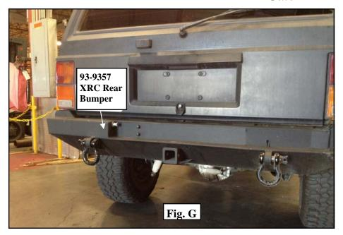
**Step 9:** Level the bumper and torque all mounting hardware according to the chart on page 15 or manufacturers specifications.
