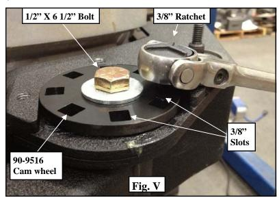
Step 34: Torque the previously installed 1/2" X 6 1/2" bolt to 80 ft./lbs. (Fig. V)
