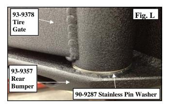
**Step 20:** Slide the main pin (90-4536) down through the hole in the rear bumper, stainless pin washer(s), tire gate, and into the lower bumper. Do not tighten at this time. (Fig M) **NOTE: The pin will be installed with the reduced shoulder on top.**
