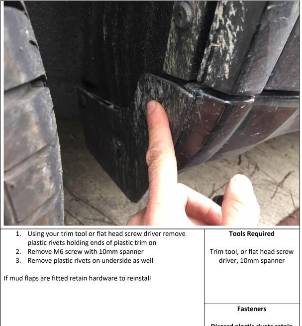
Discard plastic rivets retain any bolts/screws
