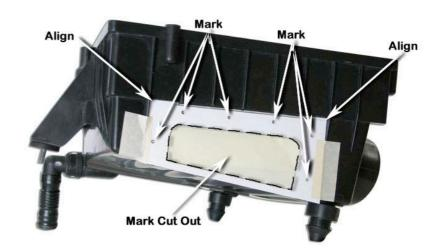
Drill a pilot hole for each of the marked hole positions.
