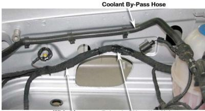
Wiring Loom Relocated Mounting Hole
