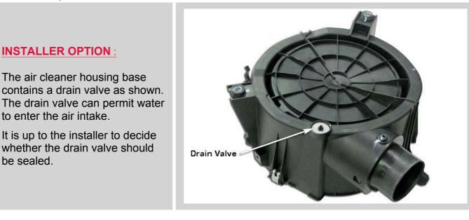
Loosely install a 70/90mm hose clamp (Item 11) over the air cleaner inlet adaptor, install the air cleaner base into the vehicle and fasten with standard mounting bolts. 70/90mm Hose Clamp
